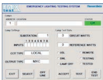
EMEX TS power units include integral touch screen monitor
